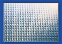
**INSIDE** - (shown above) Ripstop inside to mitigate tearing.
